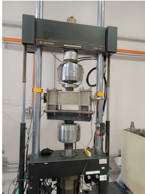
Figure 9: Double shear loading of MKI assembly by Instron testing machine
