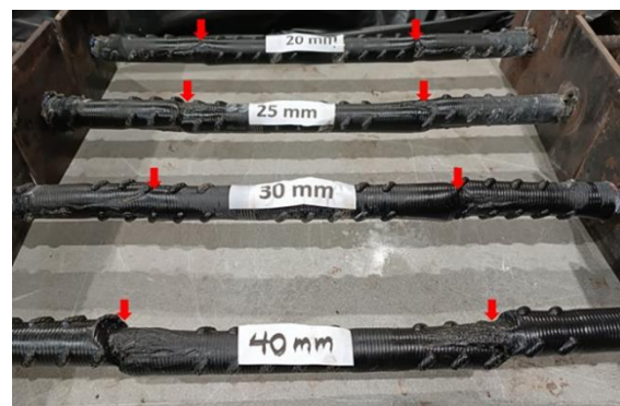
Figure 10: (a) The load – displacement graphs of samples for shear testing and (b) post-test observation of the sheared bolt sleeves at 20, 25, 30 and 40 mm.
