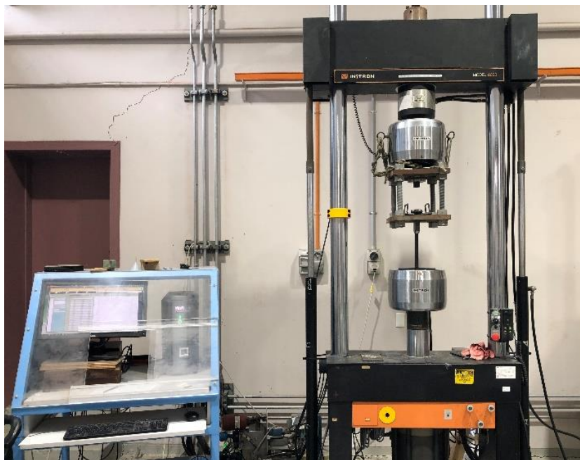
Figure 13: Test set-up for dome plate deformation test.
